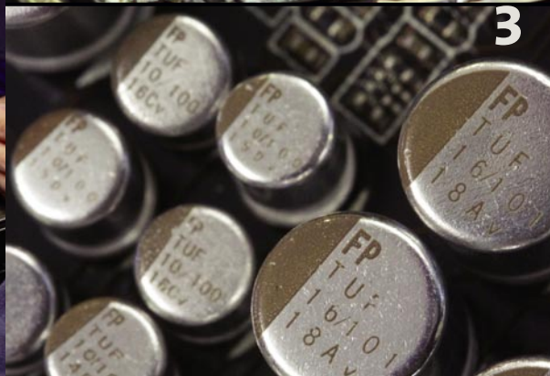
[1] Professor McKinney shows Aishish Baiju '15 the interior of the new PC's cabinet. [2] Before applying the heat sink, McKinney locks the processor into position. [3] The capacitor bank on the motherboard, part of the voltage regulator.
